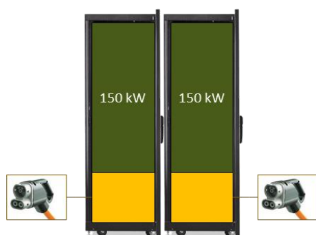
Abb. 31: Modulares System 2 x 1 x 150 kW
